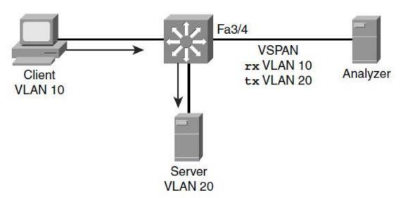
The Flow diagnostic flowing between a server in VLAN 20 and a client placed in VLAN 10
