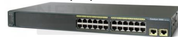
1 rack unit (1U)
