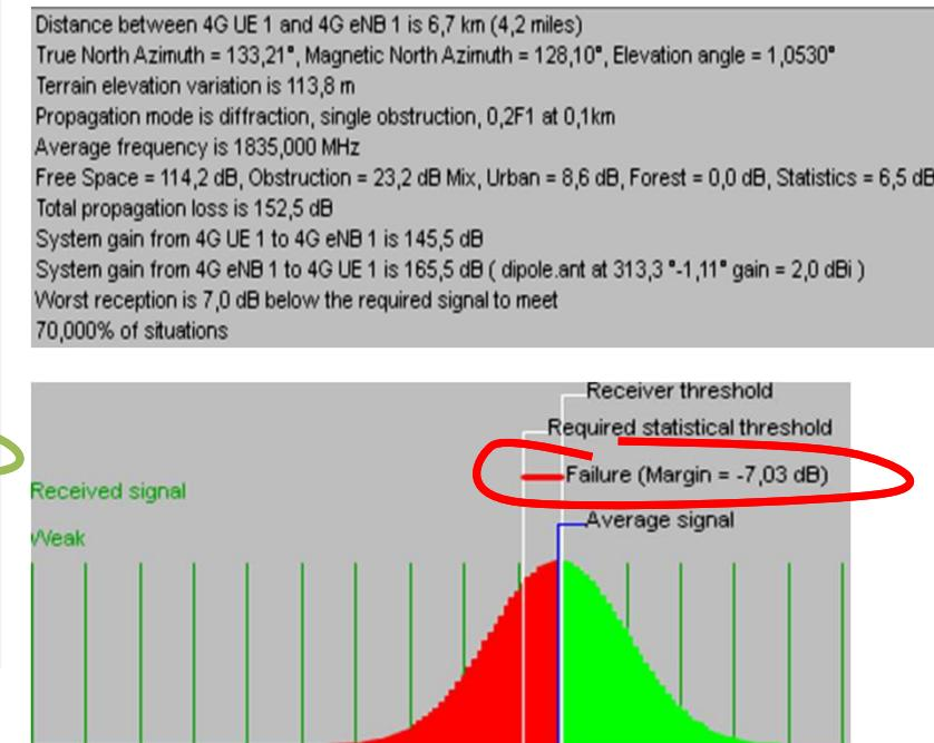
$$22.5 \text{ (EIRP)} - 114.2 \text{ (free space)} - 23.2 \text{ (obstruction)} - 0 \text{ (forest)} - 8.6 \text{ (urban)} - 6.5 \text{ (stat)} - 2 \text{ (UE line loss)} + 2 \text{ (ant.gain)} = -130 \text{ dBm}$$
