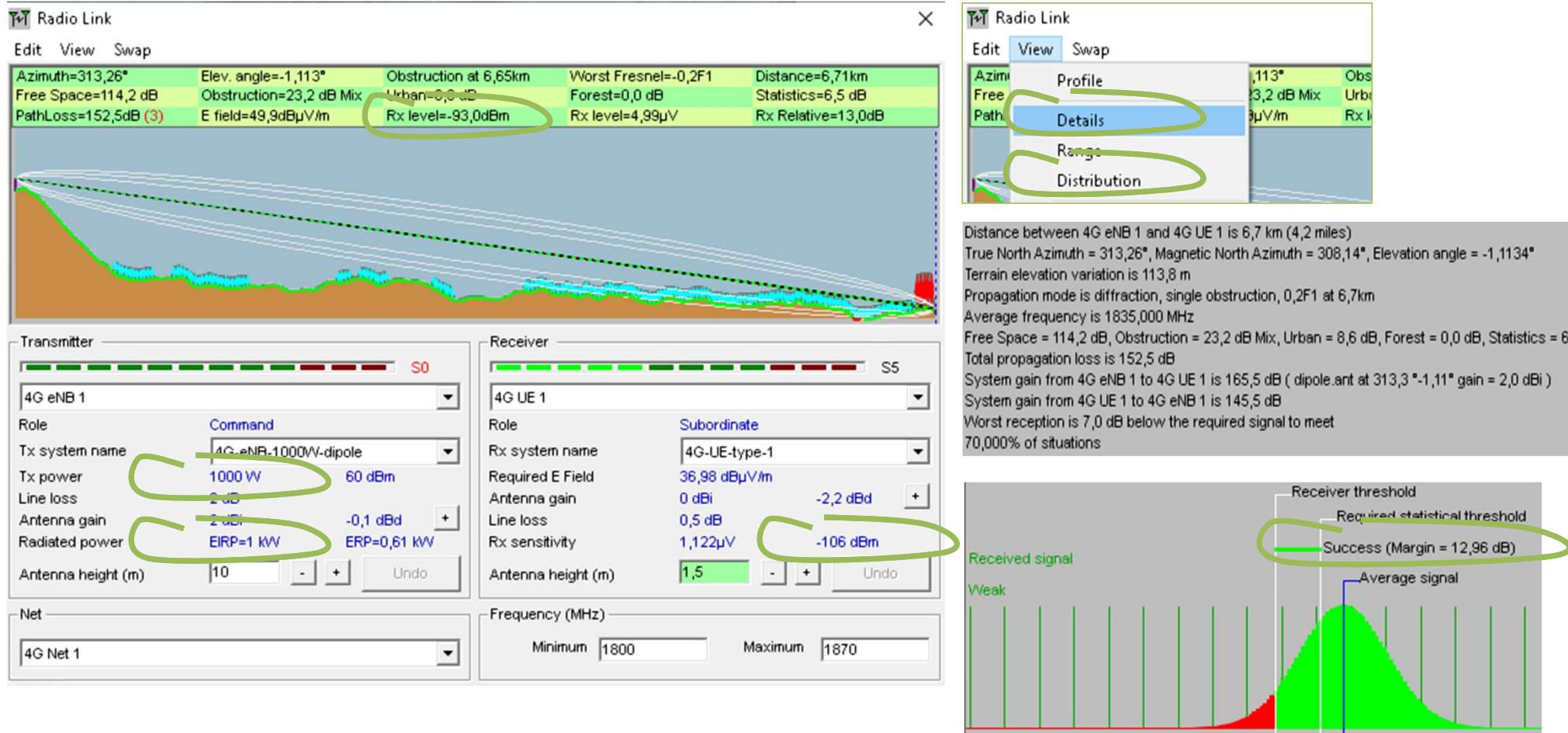
$$60 \text{ (EIRP)} - 114.2 \text{ (free space)} - 23.2 \text{ (obstruction)} - 0 \text{ (forest)} - 8.6 \text{ (urban)} - 6.5 \text{ (stat)} - 0.5 \text{ (UE line loss)} = -93 \text{ dBm}$$
