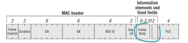
**Beacon** broadcast frames - contains all the information about the network. Beacon frames are transmitted periodically by AP, they serve to announce the presence of a wireless LAN with its capabilities – Basic Service Set support
